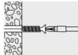
**3** Place Screw in Plug & tighten until secure
